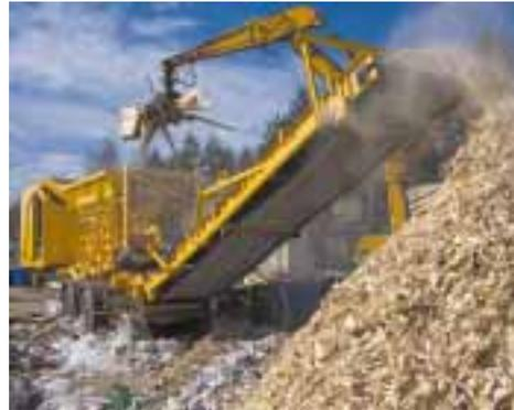
The versatility of the TANA Shark makes it possible for a customer to invest in one shredder unit that allows a quick and cost efficient conversion to suit most waste fractions. The TANA Shark may be used either as a primary shredder only or to process the material into an end product as required. It is available as a single or a twin rotor model. The investment or efficiency is not compromised in spite of changes in waste material types or contracts.
